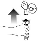
2. Open the taps completely after making the hose connection to check for water leaks at the connection points. If any leaks occur, turn off the tap and remove the nut. Retighten the nut carefully after checking the seal. To prevent water leakages and damages caused by them, keep the taps closed when the machine is not in use.
